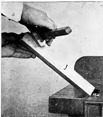
Fig. 50—Drawing Gauge Line
